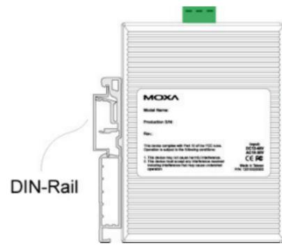
To remove Moxa EDS-205 from the DIN rail, insert a flat-blade screw driver horizontally into the DIN-rail kit under the EDS-205, and then pull it upwards and release the EDS towards you and away from the DIN rail.
