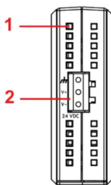
1. Heat dissipation orifices
