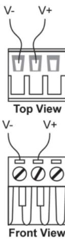
Grounding and wire routing help limit the effects of noise due to electromagnetic interference (EMI). Run the ground connection from the right most contact of the 3-contact terminal block to the grounding surface prior to connecting devices.
