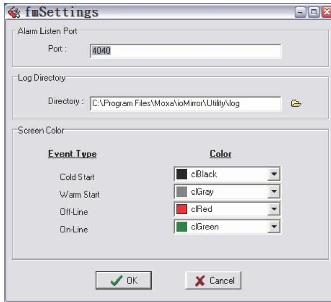
The **Alarm Listen Port** is the TCP port number that will be monitored for status events. You can modify this setting as necessary to receive signals through a firewall. It will need to match the settings for the ioMirror server that is being monitored.
