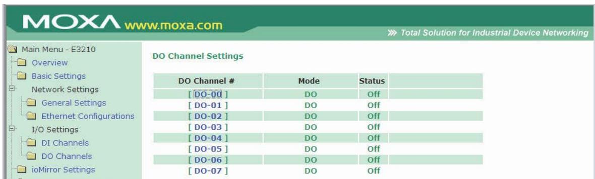
The Current Setting sets the channel's current output status in order to test the DO connection. The Power On Setting sets the channel's output status when the I/O server is first powered. The Alarm Status Setting sets the channel's output status when the I/O server is in an alarm state. The alarm is configured on the **ioMirror Settings** page. After changing the DO channel settings, do not forget to Save/Restart your system.
