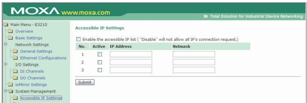
On the Accessible IP Settings page, you may control who has configuration access to the ioMirror by entering the permitted **IP Address** and **Netmask**. When the accessible IP list is enabled, only network hosts on the list may configure the ioMirror. Use the accessible IP list as follows:
