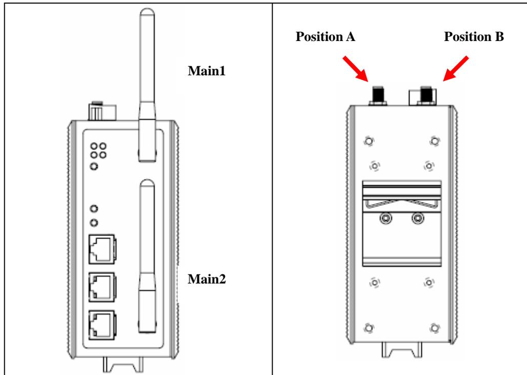
If you need to improve the performance of the Main1 and Main2 antennas, you can connect additional antennas to the side panel of the AWK-5222 using an antenna cable (Position A: AUX1 and Position B: AUX2). The default antenna for the AWK-5222 is a 2 dBi, dual-band omni-directional antenna, RP-SMA (male).
