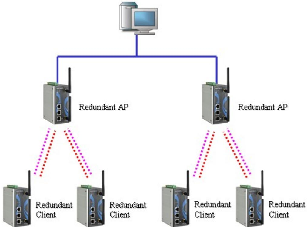
The following figure shows the Wireless Redundancy operation mode:
