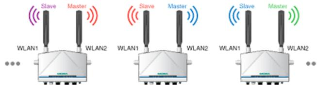
⚠ WLANs with same color must have identical RF type, SSID, and security settings.
