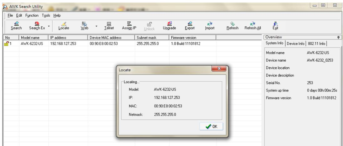
Make sure your AWK is **unlocked** before using the search utility’s icons setting. The AWK will unlock automatically if the password is set to the default. Otherwise you must enter the new password manually. Go to **Tools → AWK login Options** to manage and unlock additional AWKs.
