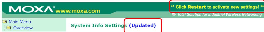
To make the changes effective, click **Restart** and then **Save and Restart** after you change the settings. About 30 seconds are needed for the AWK-6232 to complete its restart process.
