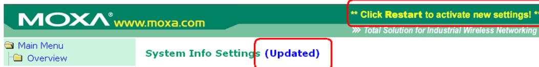
To make the changes effective, click **Restart** and then **Save and Restart** after you change the settings. About 30 seconds are needed for the AWK-5232 to complete its restart process.
